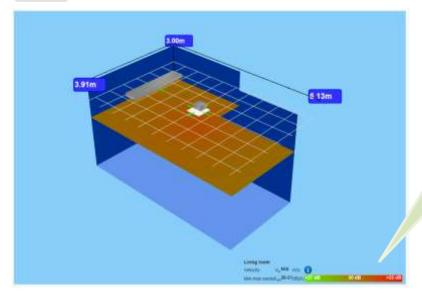
Note: The colors of the Soundview mesh are interpreted according to the sound legend at the bottom right corner
