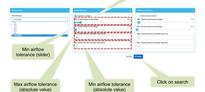
You enter the values of max and min tolerance for flow rate or pressure rate by either adjusting the slider, or entering absolute tolerance values in the corresponding boxes
